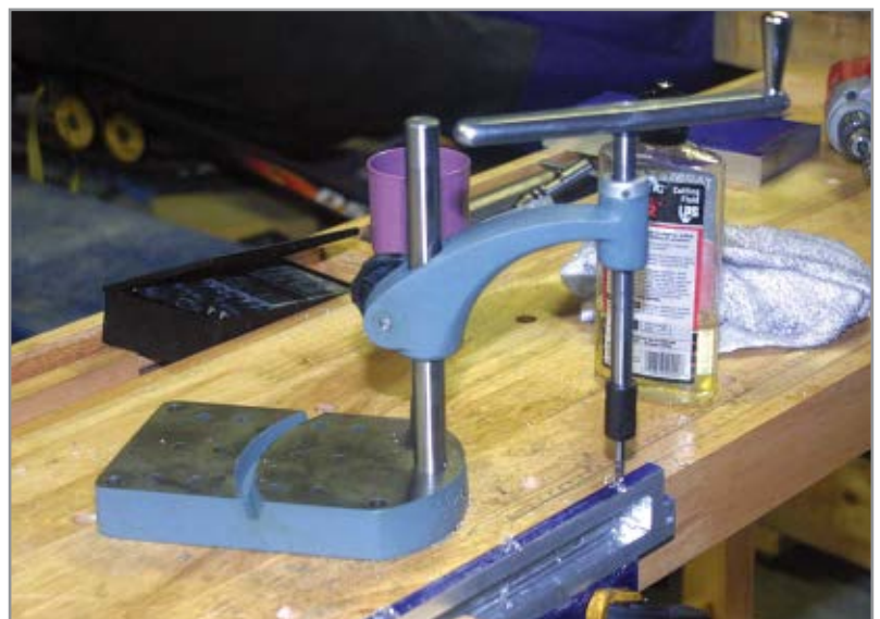
FIGURE 5. A hand tapper is used so that the tap always remains perfectly upright and in line with the hole.
