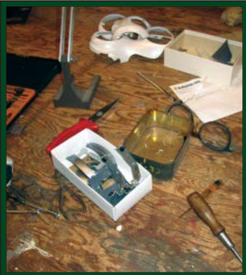
This image shows two boxes with parts from a disassembled Aibo and additional parts in white in the background. The Northern Bites team had to remove all these to get at the robot's neck, to remove it.
