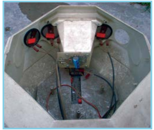
Both IR sensors and sonars (before cleaning).
