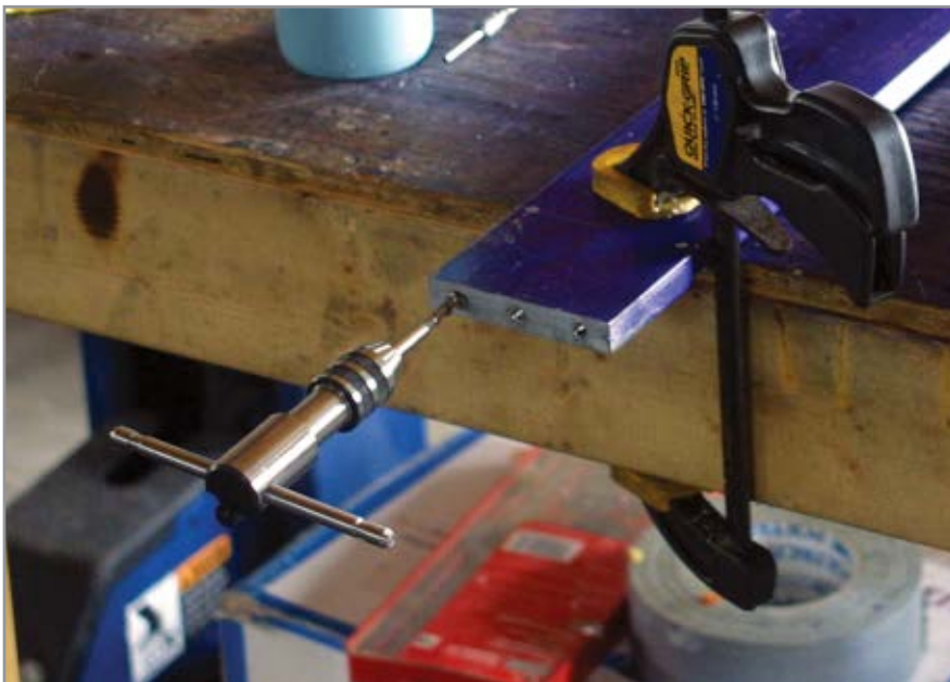
FIGURE 4. A t-handle and 1/4-20 spiral flute bottoming tap is used to create a blind hole in aluminum.
