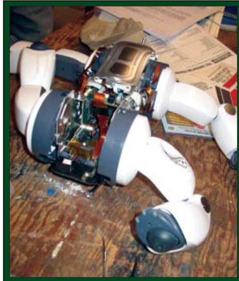
Not from Sleepy Hollow , but a headless Aibo none-the-less. On its back are silver touch-sensitive LEDs. Inside are its motors and microprocessor.
