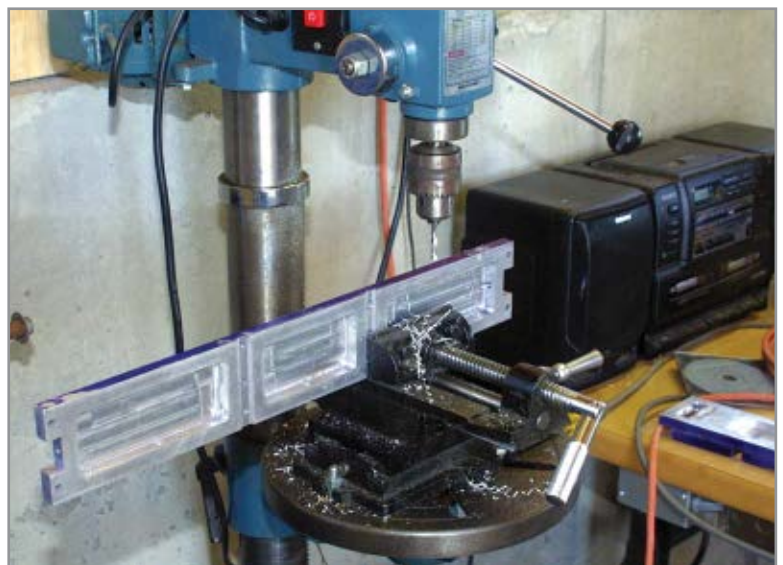
FIGURE 2. A drill press is used to make perfectly perpendicular holes in a frame rail.
