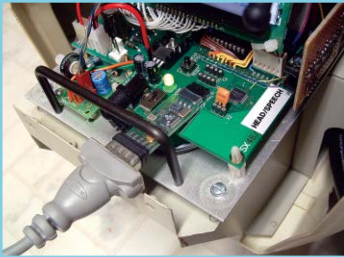
New firmware loaded on co-processor (also mounting of footlight driver).
