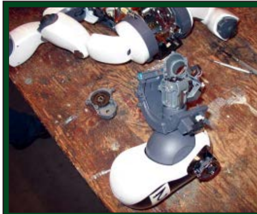
Here you can see the neck joint under repair. In the middle of the neck, on the light gray plastic is a fitting that connects the gear above the neck. The fitting has begun to erode. The team used epoxy to strengthen the connection between the gear and fitting.
