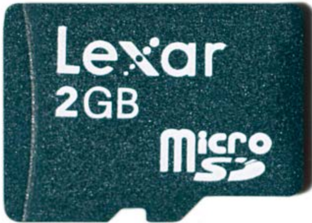
PHOTO 1. The 2 GB microSD memory card fits neatly into an automatic release microSD socket on the other side of the uDrive-uSD-G1 printed circuit board. You may also use a 64 MB or 1 GB microSD memory card if 2 GB is overkill for your application.
