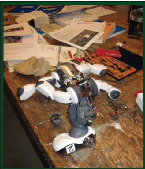
This is another disassembled Aibo with the neck removed. The gearbox was at issue here, which the team was trying to repair. It is lying left of the Aibo's head. A workbench with tools and instructions for dismembering Aibo lay in the back.
