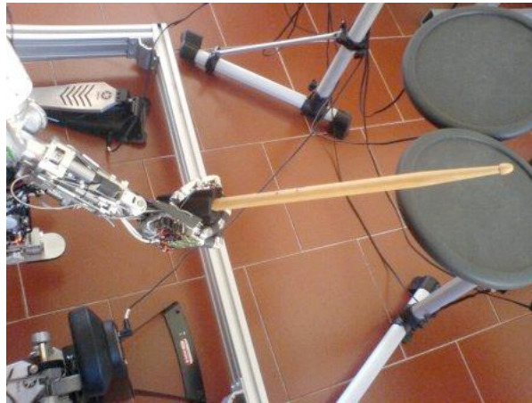
Fig. 2 iCub grasping the drumstick, and hitting the drum pads
