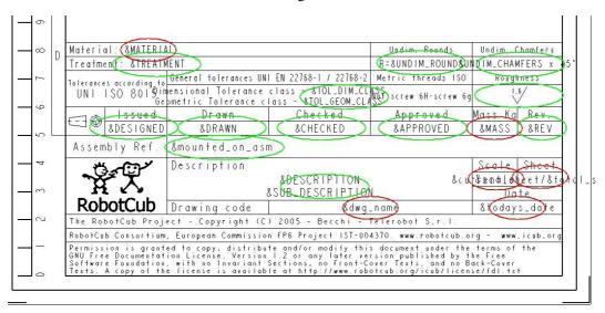
The values highlighted in red are automatically filled in by the system:
