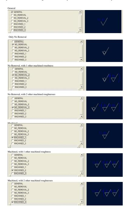
In all cases the symbol must be completed before its insertion with the "Var text" value. For roughness symbol in the drawing, the Pro/ENGINEER standard symbol ("isosurftext.sym") in the "System Sym" directory should be used.
