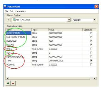
As described before, the parameter highlighted in green are defined by the user. The red ones are defined by the system at the first regeneration. Note: the MASS parameter is automatically calculated by the system as a sum of all the parts mounted in assembly in every regeneration of the model.
