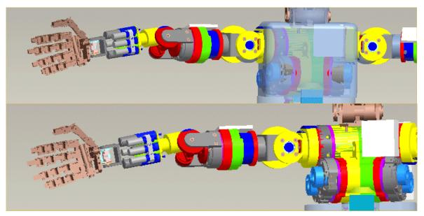
Figure 8: One of the latest design of the arm subsystem with and without the external shell.
