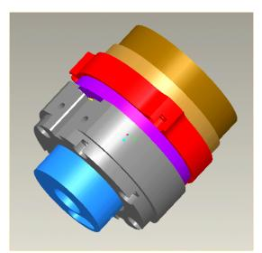
Figure 4: The Kollmorgen motor and Harmonic Drive gearbox.
