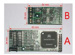
Figure 11: Left, ADC card. Right, motor controller card (A processor card, B amplifier card).
