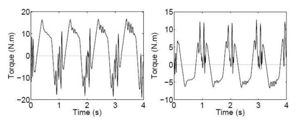
Figure 3: The left plot shows the torque applied to control the "left arm 2" joint. The right figure is a plot of the torque applied to control the left elbow.
