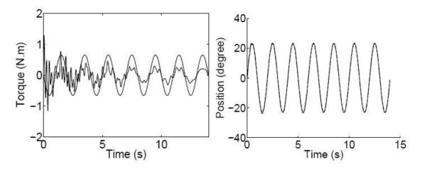
Figure 2: Torque applied to control the arm (left) and position of the arm (right). The right display contains both real position of the arm and of the desired position (input of the PID), we clearly see that they match very well (since we cannot distinguish them).
