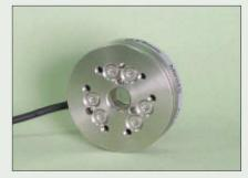
The Mini45 F/T transducer The transducer is made of hardened stainless steel with integral interface plates made from high-strength aircraft aluminum.
