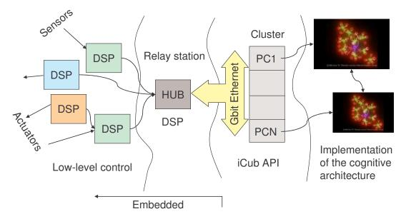
Figure 10: Levels of the hardware of the iCub.
