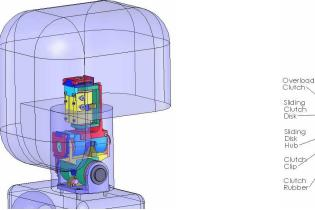
Figure 6: The neck mechanism.
