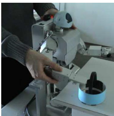
Figure 6: The demonstrator teaches the robot kinesthetically by moving the limbs of the robot.
