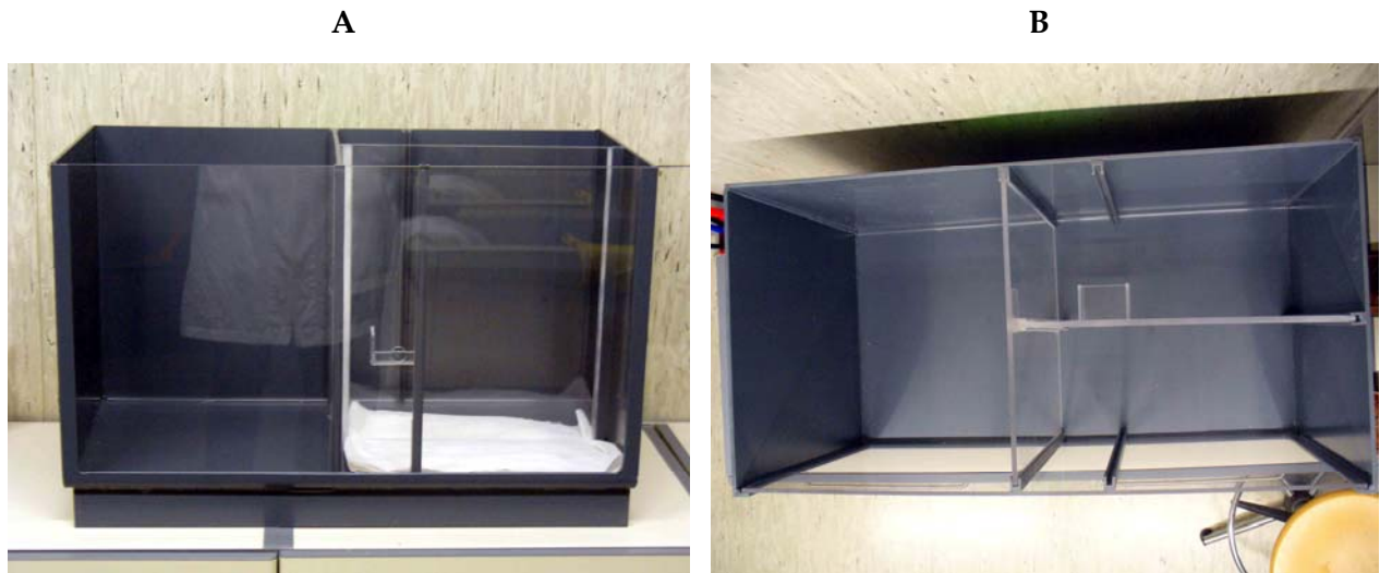
Figure 13. The cage for training and neuronal recording. A , frontal view; B , top view. The leftmost sector shown in B contains the observing rat; the lower-right sector contains the actor rat which retrieves food from the container visible in the separation.
