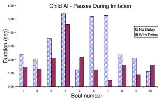
Fig. 17. The duration of pauses taken by AI during the imitation game are shortened when the robot delays its responses.
