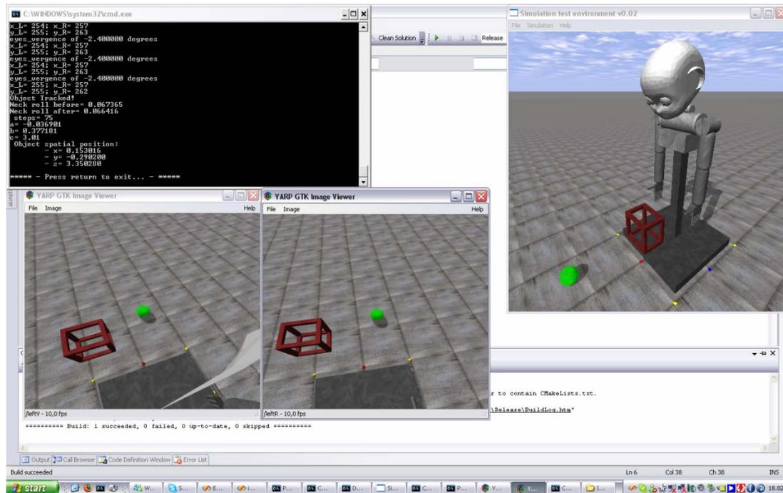
**Fig. 7** A screenshot depicting the moment in which the simulated robot tracked the position of the ball in the 3D surrounding environment. Therefore, our program uses the encoders information to triangulate the position of the centroid of the object within the simulated space.
