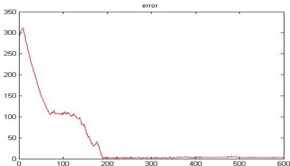
Figure 10. Error obtained with the servocontroller.
