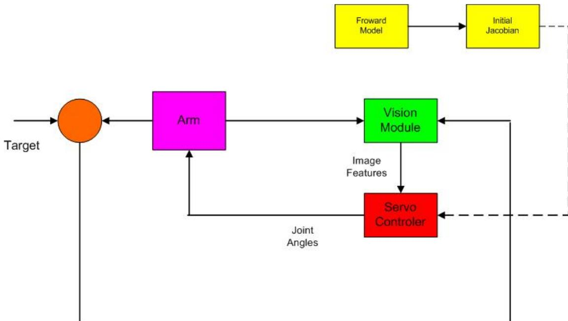
Figure 1. General Platform for the reaching based on a forward model
