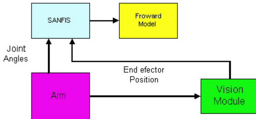
Figure 2. Calculus of the Forward model (sensory motor map) using the ANFIS
