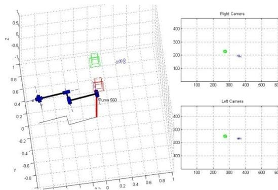
Figure 8. The left subplot has the position of the robot at the beginning of the reaching. The target position is represented by the blue points in the left subplot (feature points of the end effector at the end of reaching). The right top and right bottom subplots show the end-effector position (green circles) and the target image coordinates (blue crosses).
