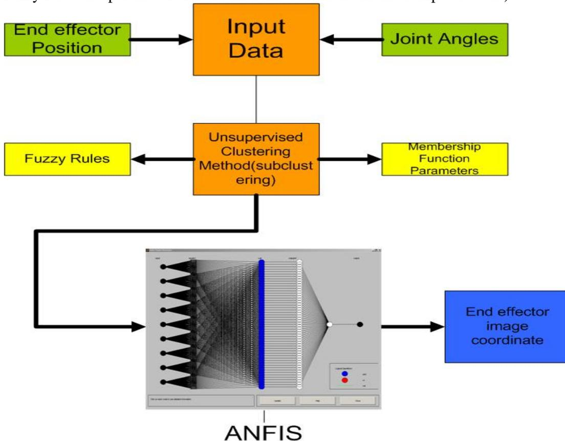
Figure 4 Construction of the forward model using an ANFIS-based methodology
