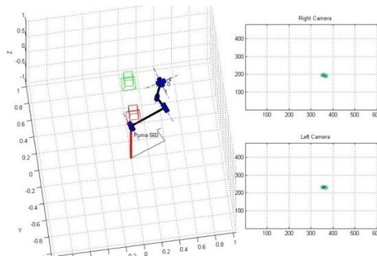
Figure 9. The left subplot has the position of the robot at the end of the reaching. The target is represented by the blue points in the left subplot (partially obscured by the end effector). The right top and right bottom subplots show the end-effector position (green circles) and the target (blue crosses). Since the robot end-effector has reached the target the blue crosses are overlapping with green circles.
