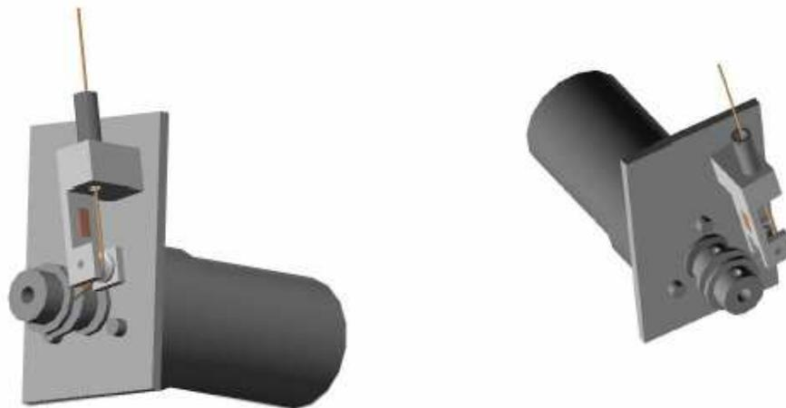
Fig. 2.2.1.4 Cable Tension Measurement using a strain gauge load element
