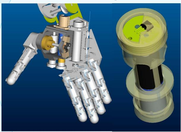
9 controlled DOF on hand finger underactuation (21 DOF in total) absolute position sensor on finger joint tension sensor on finger tendons tactile sensor (still under implementation)
