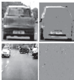
Figure 2. Top: excitation passing into the LGMD (light or dark areas) after filtering by lateral inhibition is high when an object is about to collide. Bottom: when no collision threat is present there is little excitation passing into the LGMD.
