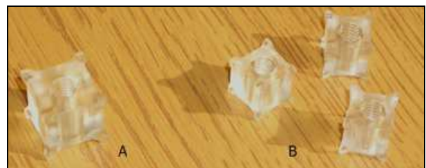
Figure 4: Coils cores: A) 12 mm transmitter triad core, B) 9 mm receiver triad cores.
