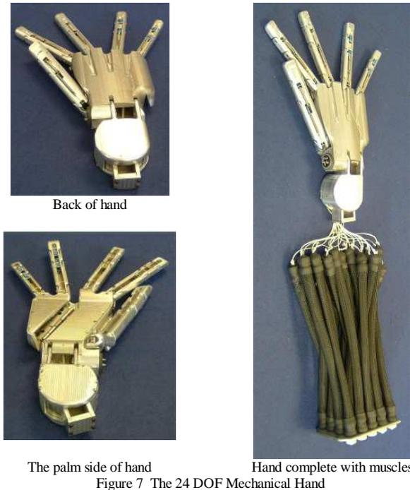
Figure 7 The 24 DOF Mechanical Hand
