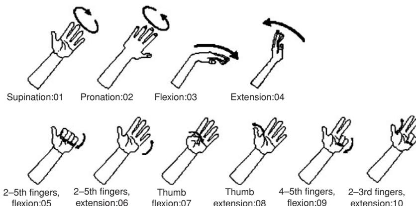
Figure 6 It shows the 10 different motions, which can be discriminated from the EMG signals (Nishikawa *et al.* 2000).
