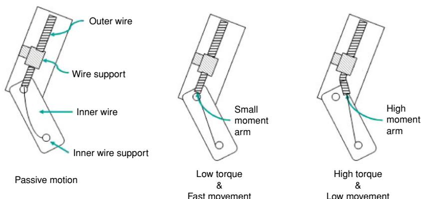
Figure 13. New adaptive torque mechanism. The spring is substituted for a spring coil outer tube. The spring coil presents similar characteristics to the spring keeping the inner wire (actuation wire) taut at all times.
