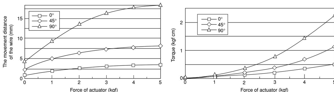
Figure 14 Statistics of the adaptive joint mechanism: (a) displacement of wire and force of the actuator and (b) joint torque and force of actuator.
