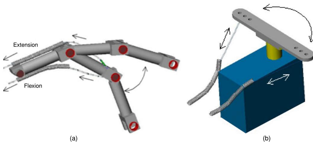
Figure 12 Adaptive joint mechanism by using spring coil type outer tube for the tendon guide. (a) The fingers' flexion/extension motion. (b) Power module by using RC servomotor.
