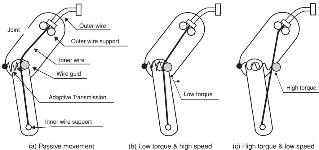
Figure 8 It shows the principle for the passive joint and adaptive torque mechanism. With light load (b) the wire is close to the fulcrum, resulting in low-torque-high-speed motion. When the load is increased (c), the wire moves away from the fulcrum, increasing the torque and reducing the motion speed (Ishikawa *et al.* 2000).
