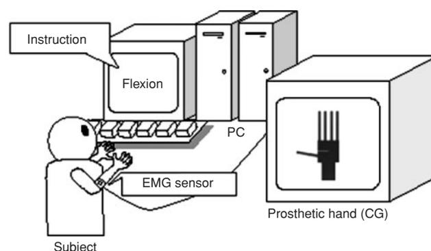
Figure 5 Experimental setup. The proposed controller is implemented in a PC. A subject pushes the keyboard to teach and watches a computer graphics hand on the monitor instead of a real-prosthetic hand as visual feedback (Nishikawa *et al.* 2000).
