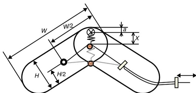
Figure 7 Adjustable power transmitting mechanism.
