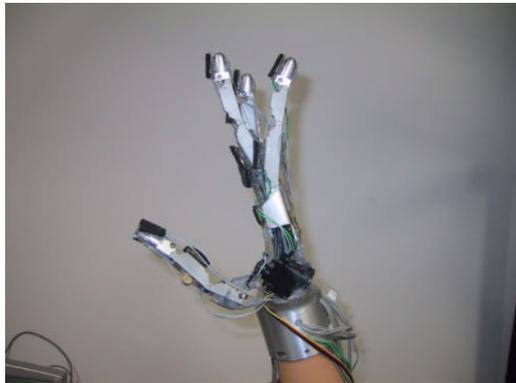
Figure 16 Aluminum body of finger part and palm part.
