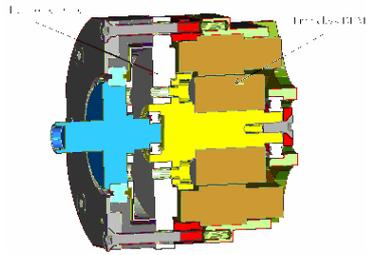
Fig. 5 View of the iCub motor/gearbox actuator group.
