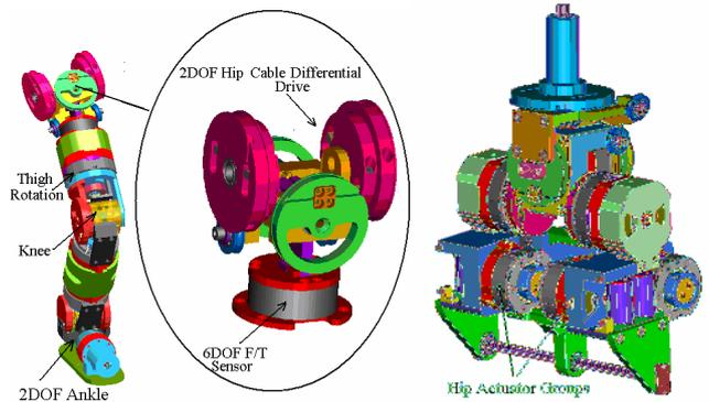
Fig. 7 Leg CAD model of the iCub and Lower torso with the housing of the hip actuators.
