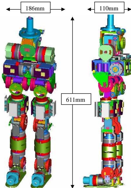
Fig. 3 CAD model of the lower body of the iCub baby humanoid robot.
