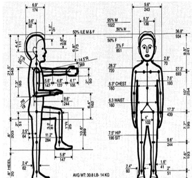
Fig. 1 Size specification for the iCub.
