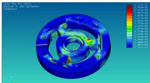
Fig. 8 The structure of the 6DOF force/torque sensor
