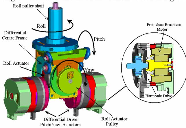
Fig. 6 The compact mechanical design of the 3DOF iCub waist.
