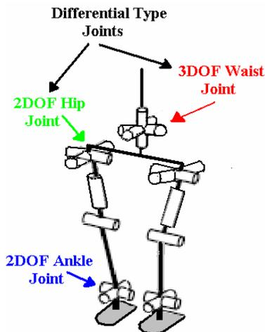
Fig. 2 Lower body kinematic configuration of iCub.
