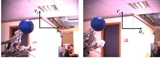
Fig. 2. Two typical images taken from the cameras mounted on the eyes of the robot (resolution  $320 \times 240$ ). The coordinates of the target (the blue ball) on the image planes will be denoted  $u_l$ ,  $v_l$ , and  $u_r$ ,  $v_r$  (respectively left and right cameras).
