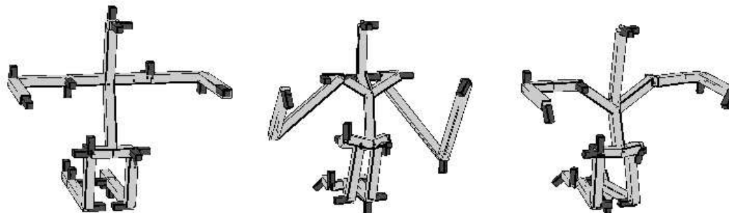
Fig. 11. Left: the Hoap3 “real” body schema, when standing on its knees. Middle: The objective body schema that was learned by the system when looking only at its hands and feet. It is not exactly the same, but the sensory relationships of both schemes (i.e., the subjective body schemes) are the same, when considering only vision of the hands and feet. Right: The body schema learned when also looking at elbows, knees, shoulders and the waist. The darker sticks indicate the rotation axis of each joint. There are three DOFs at the shoulders and the hips.
