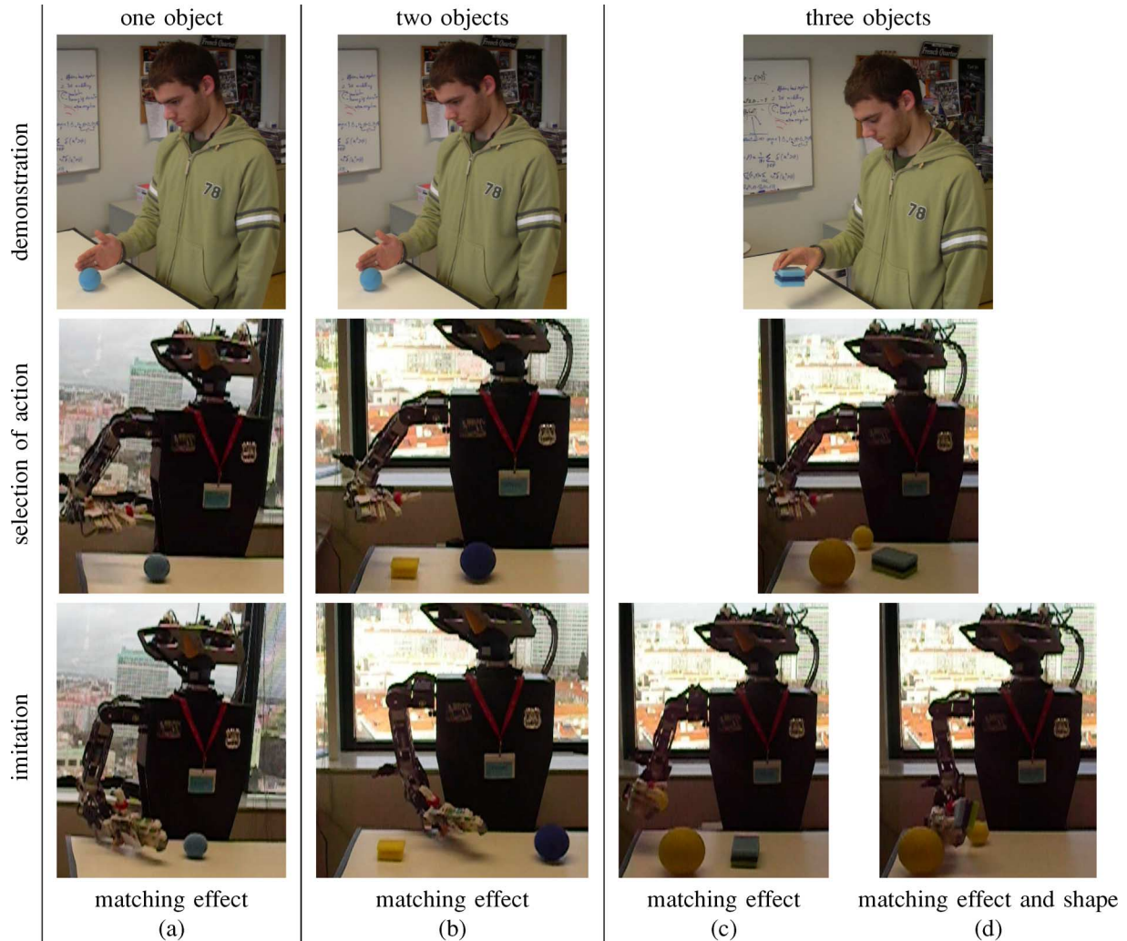
Fig. 11. Different imitation behaviors. Top: demonstration, middle: set of potential objects, bottom: imitation. Situations (a)–(d) represent imitation of actions. (a) Matching effect. (b) Matching effect. (c) Matching effect. (d) Matching effect and shape.
