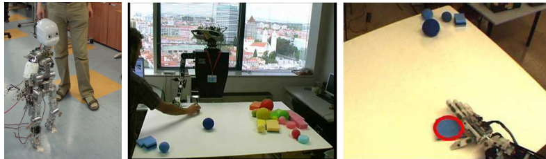
Fig. 1. Left: RobotCub humanoid platform iCub. Middle: humanoid robot Baltazar in its workspace. Right: view from one of Baltazar's eyes during a grasping task.
