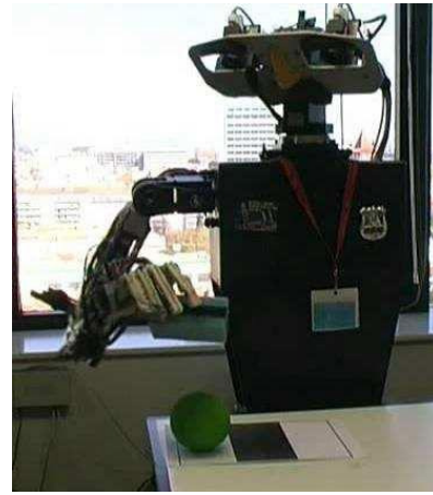
Fig. 1. Baltazar, the humanoid torso used in the experiments.
