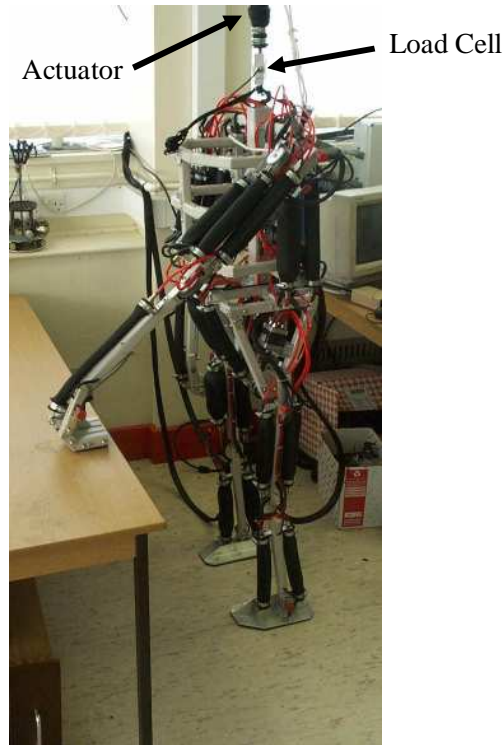
Figure 13 – Robot supported from above by force controlled hoist.
